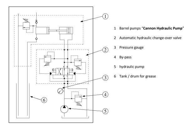
**HydMin Pump** is suited to automatic lubrication system for mobile and fixed systems where no electrical power is present. Typical such applications require that grease is pumped at pressure (for example bearings, hubs, studs, joints, etc..) in quarries, mines, industrial and manufacturing applications.
